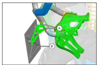
(B) - if equipped: Place the front license frame into position, then secure it with the removed M6x12 bolts (A).
