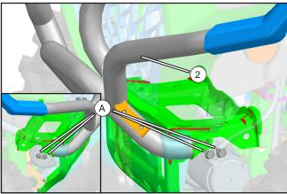
Secure the bumper end mounts to the frame with the removed M8x16 bolts (A).
