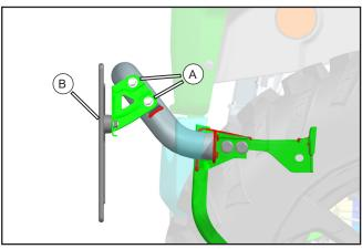
(B) - if equipped: Unscrew two M6x12 bolts (A), then take out the front license frame.
